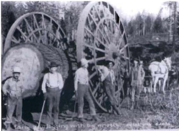
Figure 12. Early day logging with big wheels (Photo by J. H. Eastman circa 1900 courtesy Weed Historic Lumber Town Museum).
