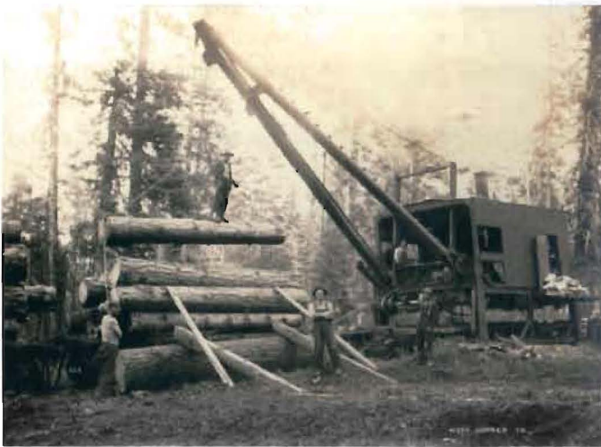
Figure 13. Loading logs with a McGiffert, 1916 (Photo by C. A. Miller courtesy of Weed Historic Lumber Town Museum).
