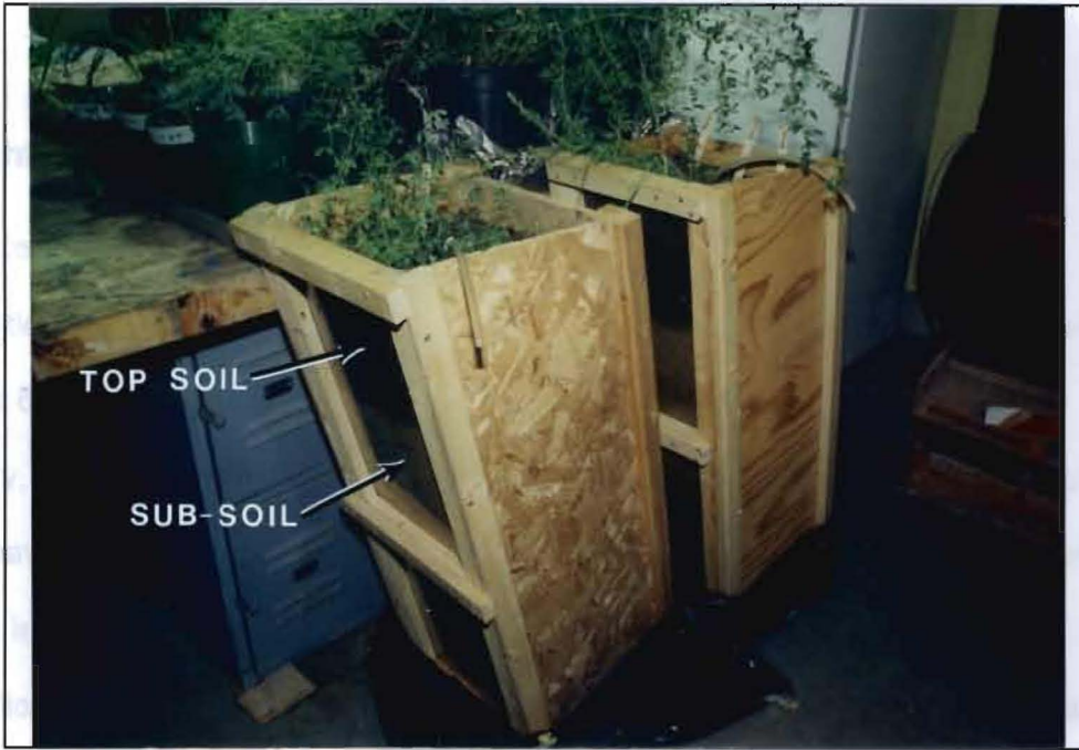
Figure A-4. Root development of Lespedeza cuneata and three species of prairie grasses. Seedlings were planted 5 cm from a 15° tilted plastic face for periodic root measurements.
