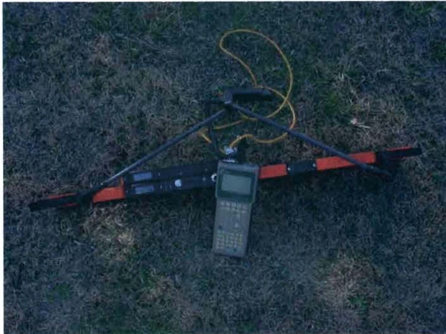
Figure 9. Geonics Limited Electromagnetic Ground Conductivity Meter Dual Output (EM-38B) with Juniper Systems Pro-4000 Data Logger.
