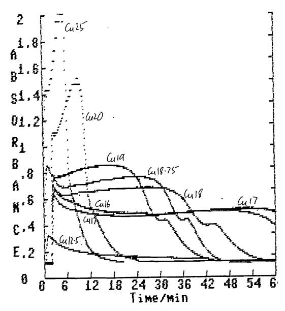
Figure 10 : The variation of absorption with time for various copper concentrations. The concentration of stock K2S2O8 is 4X10<sup>-2</sup> M
