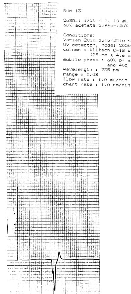
CuSD4: 1X10 - M. 10 mL 60% acetate buffer/40% methanol, 30 m Conditions: Varian 2010 pumb/2210 system UV detector, model 2050 column : Alitech C-18 cartridge (25 cm X 4.6 mm) mobile phase : 60% of acetate buffer and 40% methanol wavelength : 235 nm range : 0.08 flow mate : 1.0 mL/min
