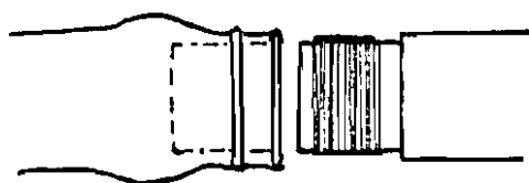
Figure 2. Tenon and socket joining of recorder and/or flute segments (Dotted lines in left segment indicate where tenon is inserted into socket.)
