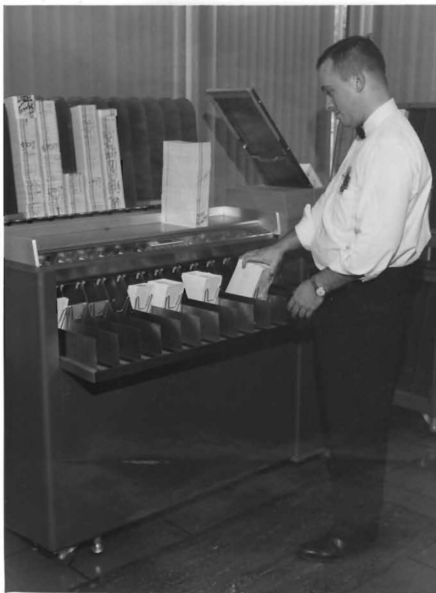
performed with consideration to time at the various points. FIGURE 10 REMOVING PUNCHED CARDS FROM THE IBM 084 SORTER ... of furniture and storage for ... to complete ... of data at ... of the computer is offered on that point ... and is made prior to the ... in 10 months.
