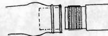
Figure 2. Tenon and socket joining of recorder and/or flute segments (Dotted lines in left segment indicate where tenon is inserted into socket.)
