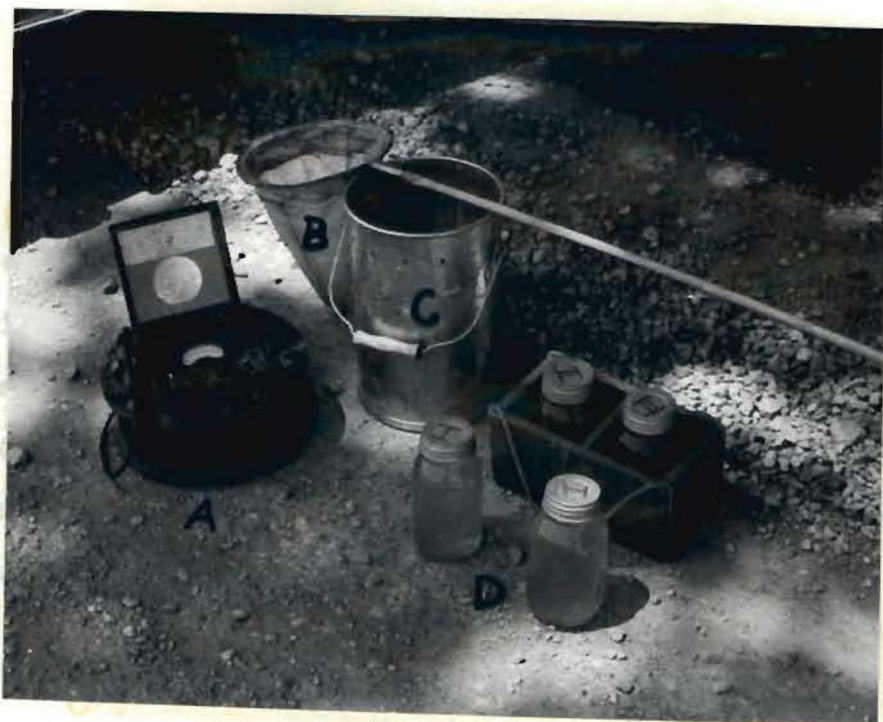
Fig. 5. Field equipment. (A) Whitney underwater electrical resistance thermometer; (B) number 20 plankton net; (C) 10-liter water bucket; (D) oxygen and carbon dioxide sampling jars.
