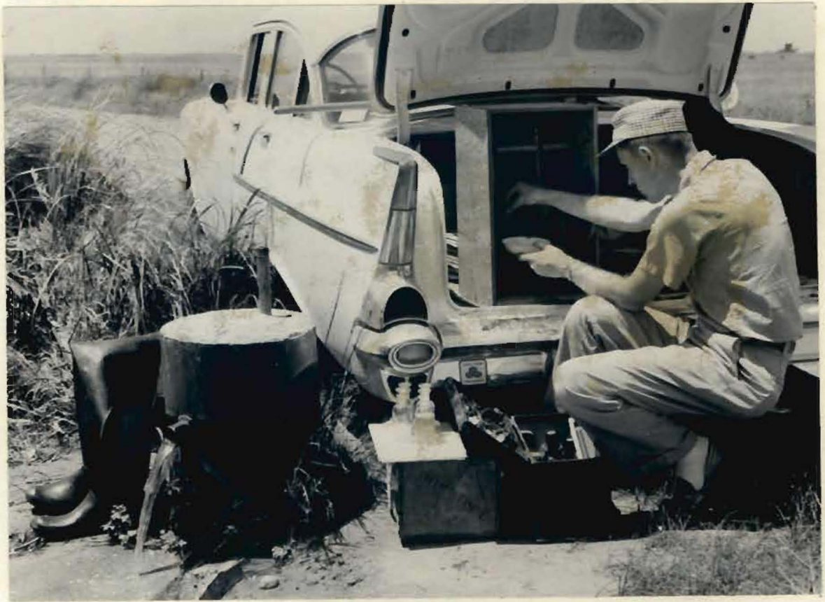
Fig. 6. Alkalinity determination using field titration unit.
