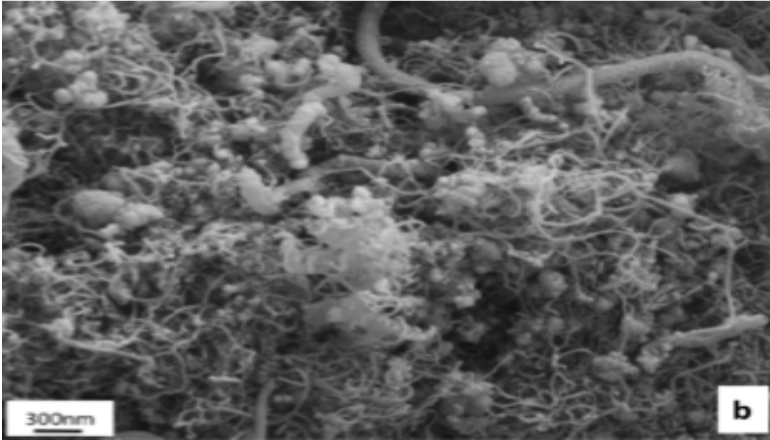
Figure 5. SEM images of Multi Walled Nanotubes (MWNTs) and Carbon Nano Fibers (CNFs) covering the surface of 5 wt % Fe loaded fly ash [22] .
