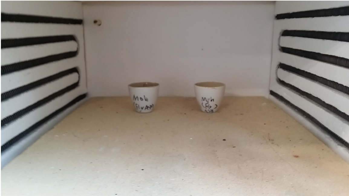
Figure 17. 2.5 (wt %) Fe loaded fly ash, after heated for 12 hours at 800 °C.
