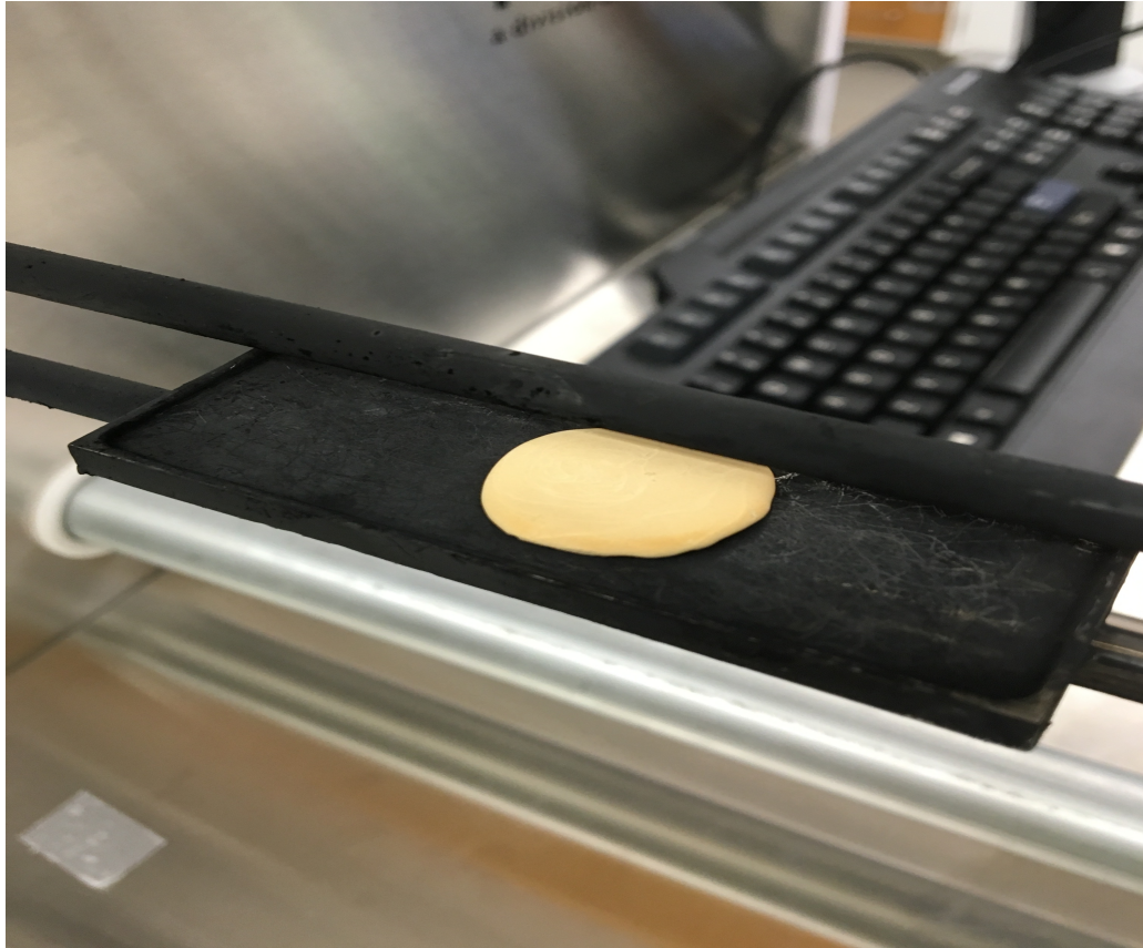
Figure 23. Sample tablet being introduced into the CVD apparatus at Kansas State University. Photo by Eric L. Trump, Ph.D., Emporia State University.
