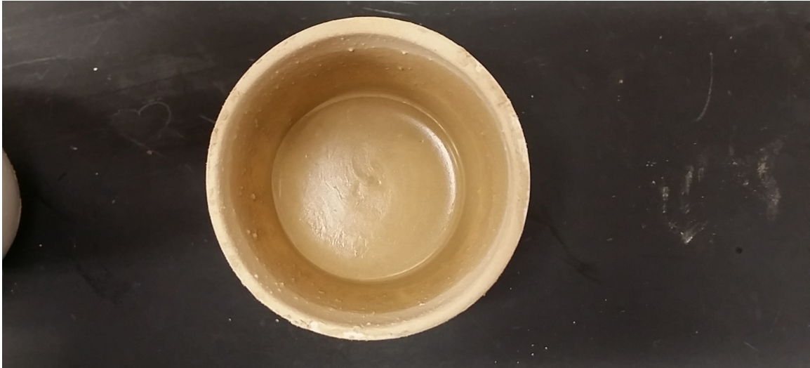
Figure 15. First sample 2.5 (wt %) Fe loaded fly ash, sandy to yellow color.
