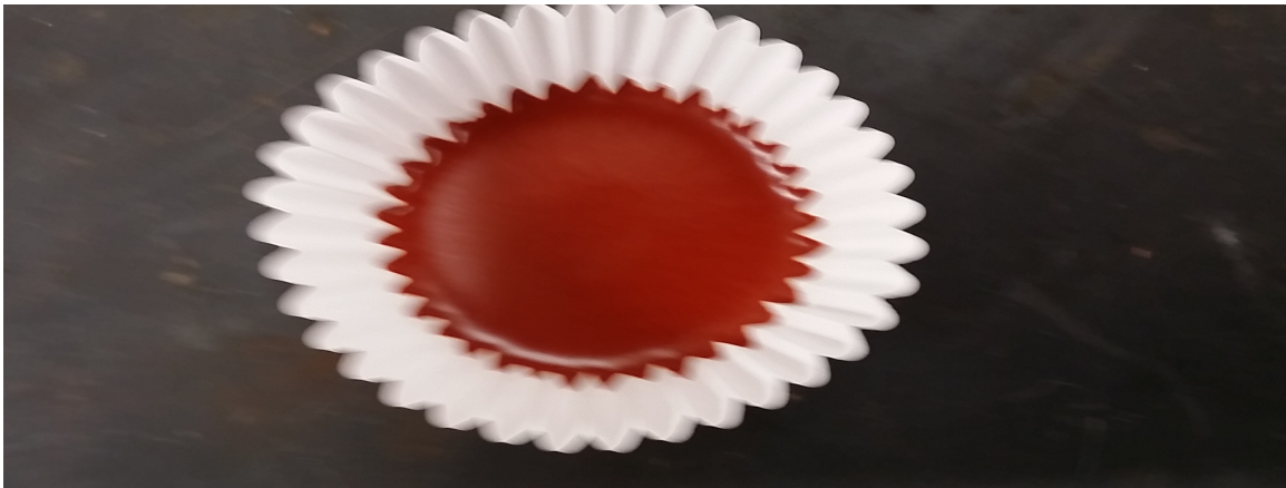
Figure 16. The second sample 20 (wt %) Fe loaded fly ash. Note the darker brown color.
