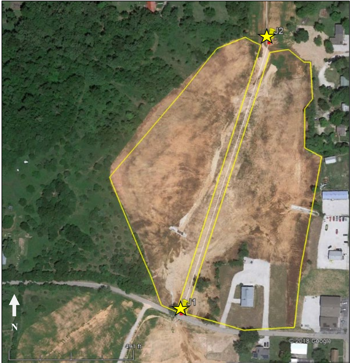
Figure 33. Study area measurement of Conduit 1 (C1). Length of C1 was measured as 348 meters (1,141 feet) (Google Earth, May 24, 2017).
