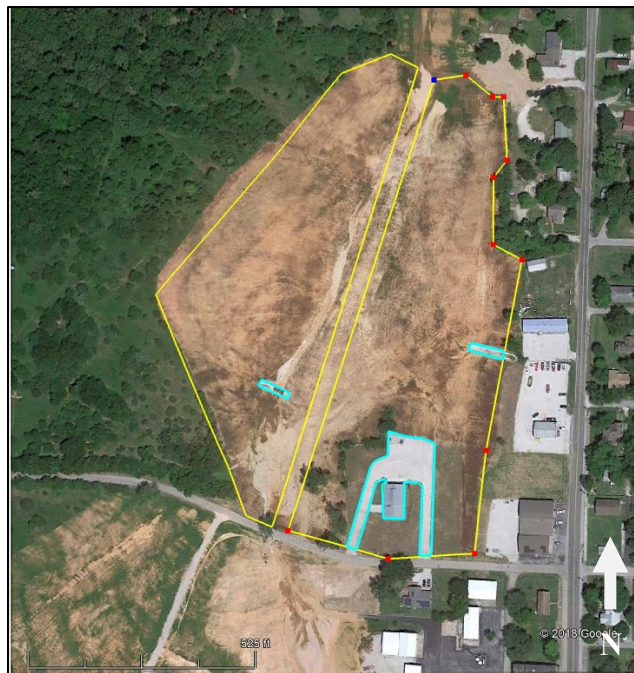
Figure 26. Post-remediation conditions, with total surface area of the west slope as the second subcatchment, referenced as S2-ESlope. (Google Earth, May 24, 2017).
