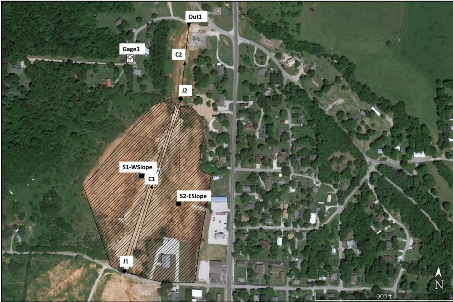
Figure 12. SWMM model area with subcatchments (S1 – West Slope and S2 – East Slope), Junctions 1 and 2 (J), Conduits 1 and 2 (C), and the outfall point (Out1). (Google Earth, May 24, 2017).
