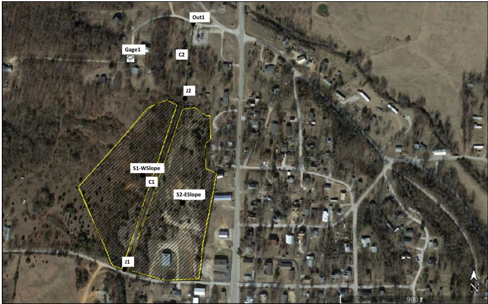
Figure 11. SWMM model area with labeled subcatchments (S1 – West Slope and S2 – East Slope), Junctions 1 and 2 (J), Conduits 1 and 2 (C), and the outfall point (Out1). (Google Earth, January 25, 2014).
