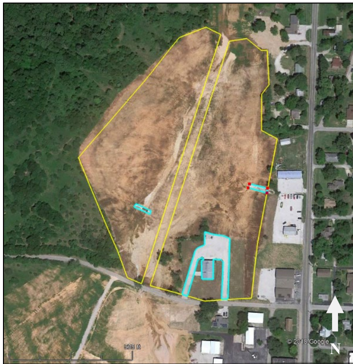
Figure 28. Post-remediation conditions, with surface area of the impervious surface of a rock diversion ditch in blue outlines on the east slope. (Google Earth, May 24, 2017).
