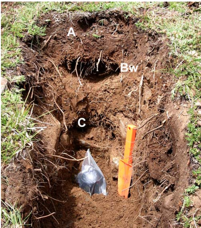
Figure 11. Soil sample pit showing soil horizons and the temperature logger at the bottom. The data logger is sealed in a plastic bag with moth balls to prevent moisture and animal damage. Digging trowel is approximately 25 cm (10 inches) long. For location see Fig. 4.
