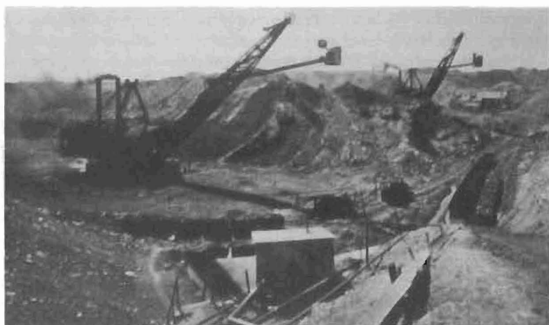
Steam shovels used in mining Crawford County coal. (Courtesy Pittsburg State University Library).
